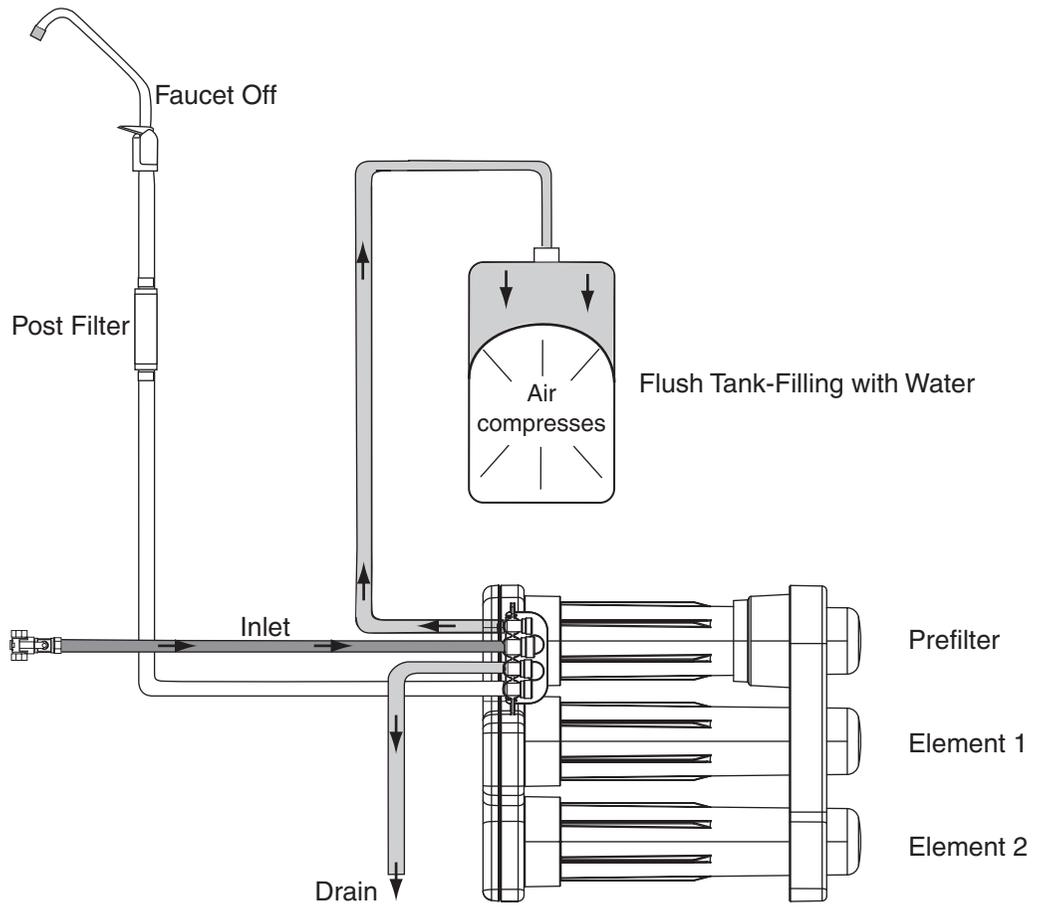
Merlin System is Producing Permeate Water for Flush
