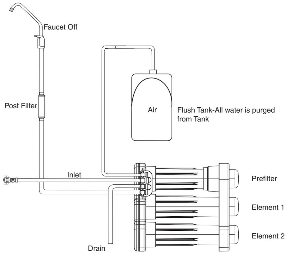
Low TDS water has flushed out the inlet side of the elements. Complete process may take 3 to 8 minutes.
